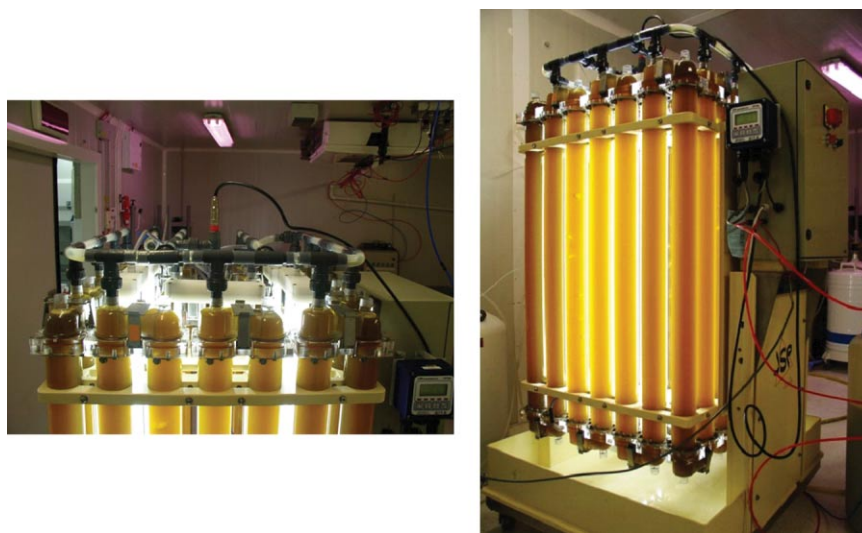
Figure 13. Photographs of the 120-L multimodule photobioreactor (top and front views). [Color figure can be seen in the online version of this article, available at www.interscience.wiley.com .]
